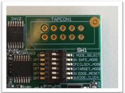
This DIP Switch is used to configure transparent and non-transparent modes, set and select the clock source.
