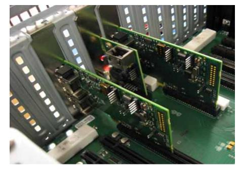
Figure 2–3 DXU405 Uplink board installed in DXE410 Chassis
