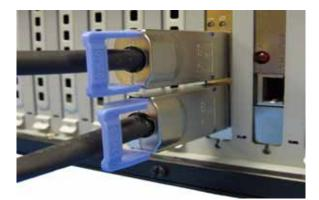
Figure 3–2 Cable Connections to Uplink board
