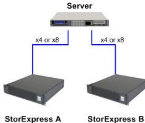
Figure 6 StorExpress Single Server Scaling Out
